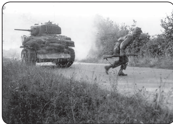
An M5 Stuart Light Tank supports US infantry. Note how it has dozer blades fitted to push through bocage hedgerows.
